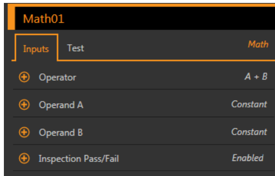
Figure 253. Math Tool—Input Parameters
