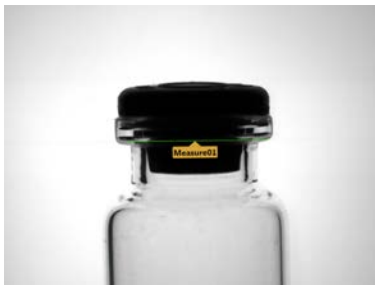
Figure 205. Measure Tool from Edge02 to Edge03
