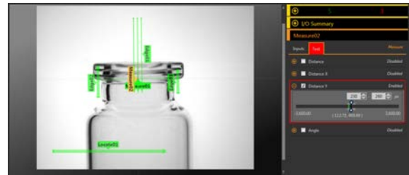
Figure 209. Bad Part—Missing Stopper
