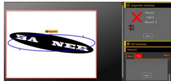
Figure 232. Bad Part—Missing Letter
