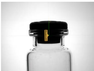
Figure 206. Measure Tool from Edge01 to Measure01
