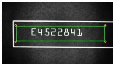
Figure 110. Light Date/Lot Code on a Dark Background
