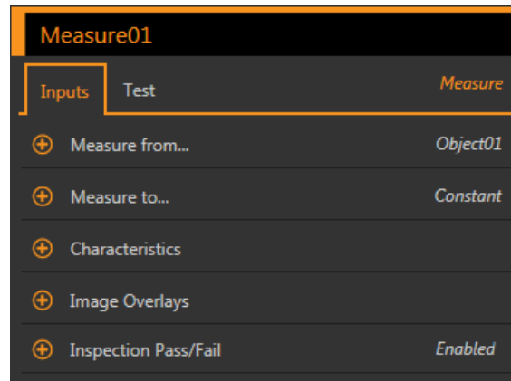
Figure 263. Measure Tool—Input Parameters
