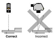
Figure 9. Orientation for a color or luster difference
