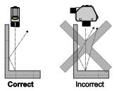
Figure 7. Orientation for a turning object
