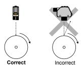
Figure 8. Orientation for a height difference
