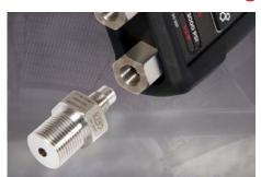
Crystal Pressure Fittings\* are machined in high-strength 316 Stainless Steel to operate at 10 000 psi/700 bar. Removable CPF adapters shift everyday thread wear away from the HPC50 Series' ports, while a self-venting weep hole alerts you before you disconnect from a pressurized system.
