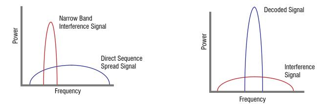
The figure above shows how the DSSS 802.11b systems filter out noise from a narrow frequency. Because of the signal processing, the Banner wireless system appears 10 dB quieter than a 802.11b radio of the same power. This means that the Banner wireless system can only interfere with 802.11b systems up to about 50 feet. Beyond 50 feet, Banner's signal is simply too low to interfere with the 802.11b system.
