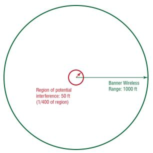
While the Banner access point (Gateway) can communicate with other Banner Nodes up to 1000 feet away, it cannot interfere at all with 802.11b devices more than 50 feet away.
