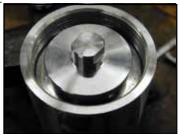
14. Install the spring and upper spring guide onto the lower spring guide.
