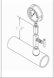
Hex gauge syphons act as thermal and liquid seal barriers between hot process vapors (such as steam and heat transfer fluids) and the gauge pressure instrument. It is designed to replace the large installation space requirements of the traditional "pigtail" syphon, providing maximum instrument protection in half the space. This reduced radius minimizes weight and deflection stress at the primary valve.
