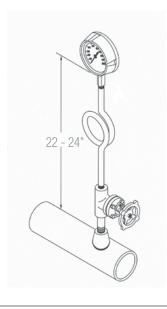
The installation can be simplified using a model HGSY gauge syphon installed in a traditional root valve. An added benefit is the reduced space envelope.
