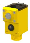
The Wireless Q45 Sensor with Button and Light as a wireless node with independently controlled push button input and a four-color LED indicator light. The push button can be configured with DIP switches for either toggle or momentary operation; the red, yellow, green, and blue LED indicator light outputs can be configured for solid or flashing operation.
