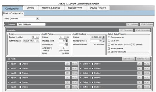
Use a USB to RS-485 adapter cable to connect a standalone DX80 Gateway to the computer. For DXM Controllers with an internal DX80 radio, connect a computer to the DXM Controller using the supplied USB or Ethernet connection. Download the most recent revisions of the configuration software from Banner Engineering's website: https://www.bannerengineering.com/us/en/products/wireless-sensor-networks/reference-library/
