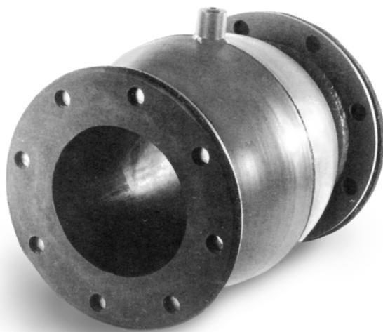
The Series 4700 Spun Aluminum Pinch valve is designed for low pressure service, in control or on/off applications. The Series 4700 is similar to the Type A, but the body is constructed of entirely of spun aluminum for weight savings and easy installation. The air actuated Series 4700 is ideal for O.E.M. accounts, Gravity Flow Applications, Pneumatic Conveying Systems and Waste Treatment Plants.
