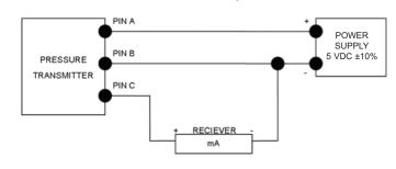
Figure C: Ratiometric Output Connection
