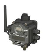
The SureCross® wireless system is a radio frequency network with integrated I/O that operates in most environments and eliminates the need for wiring runs. Systems are built around a Gateway, which acts as the wireless network master device, and one or more Wireless Q45 Sensors.
