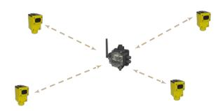
The SureCross® DX80 wireless I/O network provides reliable monitoring without the burden of wiring or conduit installation. The SureCross wireless network can operate independently or in conjunction with a Modbus host system, PLC, and/or PC software. The SureCross DX80 network is a deterministic system—the network identifies when the radio signal is lost and drives relevant outputs to user-defined conditions. Once the radio signal is reacquired, the network returns to normal operation.
