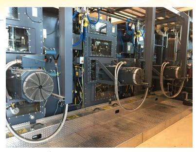
Replacing a defective fan before catastrophic failure saved about two days of production time.
