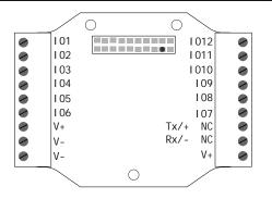
IOx. Input or output (depending on configuration)
