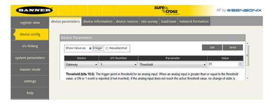
To define which of the 12 I/O points are outputs for the selected device, adjust the threshold parameter for I/O point 9. In the example below, bits 11 through 5 are used to set seven outputs (1111 1110 0000 = 0x0FE0 = 4064)
