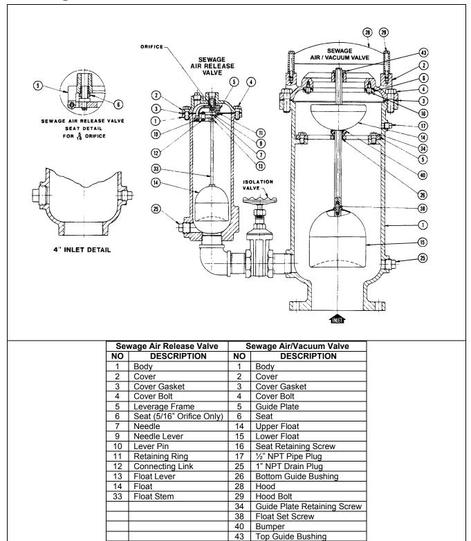
Figure 1: ASD-400C Part Identification-Sizes 4" through 14"
