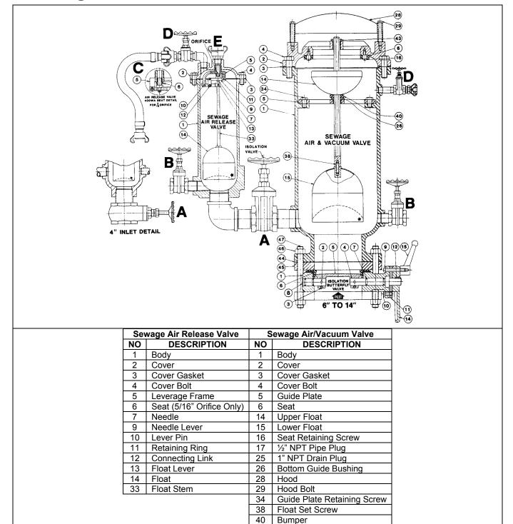
Figure 3: ASD-400C with Attachments-Sizes 4" through 14"
