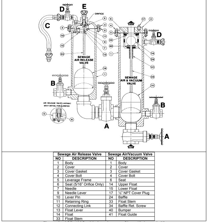
Figure 2: ASD-400C with Attachments-Sizes 1" through 3"
