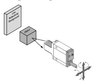
The sensing energy of a convergent mode sensor is concentrated at the specified focus point. Convergent mode sensors are less sensitive to background reflections, compared with diffuse mode sensors. However, if background reflections are a problem:
