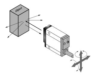
If the Alignment LED does not turn OFF when the object is removed from the beam, the sensor is probably detecting light reflected from some background object. To remedy this problem:
