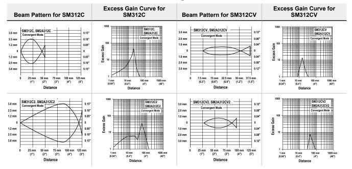
Performance is based on a 90% reflectance white test card.
