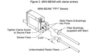
1. Prepare the sensor ends of the fibers (see Cut the Plastic Fiber on page 5).
