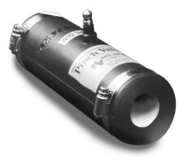
The Red Valve Type R Air Actuated Pinch Valve is 100% full ported bidirectional valve designed for tough slurry applications. The elastomer sleeve closes on entrapped solids in the line. The flexing action of the sleeve breaks any sediment or build-up in the valve, which makes the Type R rellable low maintence value
