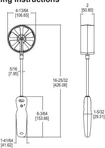
The **Model VP2 Wireless 100 mm Vane Thermo-Anemometer Probe** measures air velocity, air flow, humidity, and temperature when combined with Models UHH and UHH2 or the Dwyer Mobile Meter app. By having a larger diameter, the rotating vane is able to measure velocities down to 50 fpm or 0.25 m/s. An arrow is molded into the vane housing to depict the flow direction.
