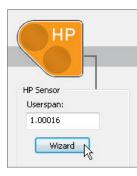
Userspan Wizards remove the effort of calculating the userspan value by allowing you to enter two calibration points (typically the midpoint and full scale values), and calculate the userspan for you. The wizard can optionally read the displayed value directly from the Model 30 when you enter is the applied pressure. To use the Userspan Wizard, simply click the appropriate *Wizard button* and follow the on-screen directions.
