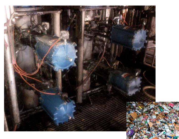
Four 8" (200mm) DeZURIK KGC-MD Maximum Duty Knife Gate Valves are installed in two High Density (HD) Cyclone Cleaners at a recycle paper mill. These valves lasted three times longer than the previous valves installed in this service.
