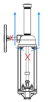
Figure 4- Knife Gate Valve with Bevel Gear Actuator, Vertical Lifting
