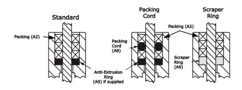
Figure 3—Packing Ring Detail
