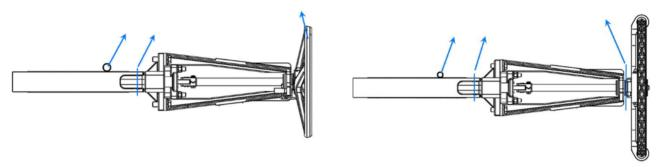
Figure 3, Knife Gate Valve with Handwheel or Chainwheel Actuator, Horizontal Lifting
