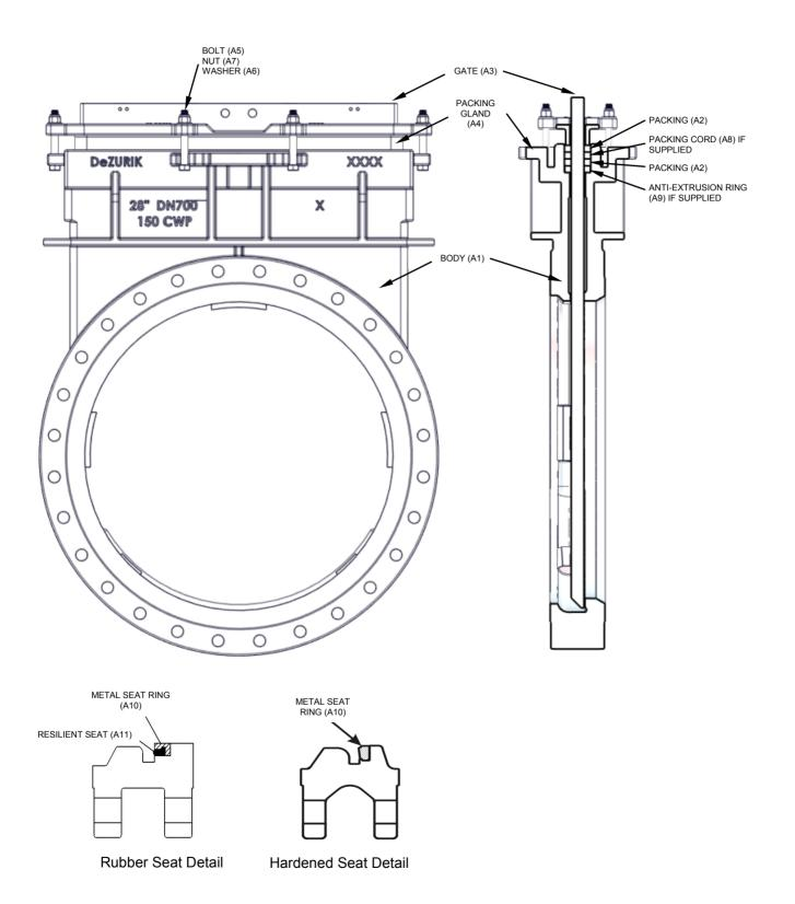
Figure 2—Component Identification
