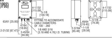
The SERIES 616WL Differential Pressure Transmitter senses very low pressures of air and non-combustible, compatible gases and sends a standard 4-20 mA output signal. All models, including those featuring the 3 digit LCD digital read-out, are factory calibrated to specific ranges as listed in the chart below.
