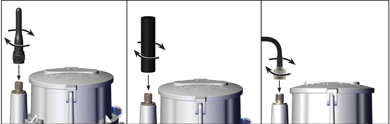
Figure 4. Attaching the cellular antenna
