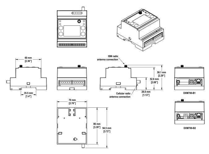
All measurements are listed in millimeters [inches], unless noted otherwise.
