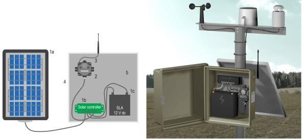
Figure 2. Example solar-powered weather station application
