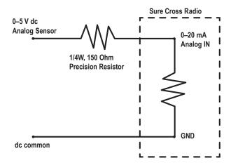
Example 1 - Converting a 0–5 V dc sensor output
