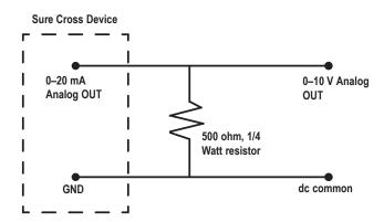
2. Connect to the same Analog OUT and GND (dc common/ground) connections in the terminal block.
