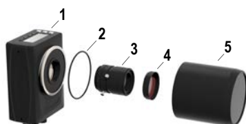
Illustration 3. Installation des accessoires
