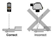
Figure 10. Orientation for a color or luster difference
