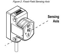
In the drawings and information provided in this document, the letters E, R1, and R2 identify how the sensor's three optical elements (Emitter "E", Near Detector "R1", and Far Detector "R2") line up across the face of the sensor. The location of these elements defines the sensing axis, see Figure 2 on p. 2. The sensing axis becomes important in certain situations, such as those illustrated in Figure 5 on p. 3 and Figure 6 on p. 3.
