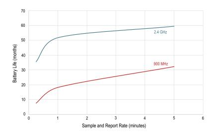
Figure 8: Battery life for the Q45UA
