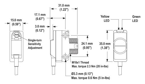
Figure 12. Dimensions for each connection type
