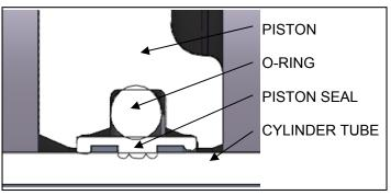
Figure 4—Piston Seal Detail
