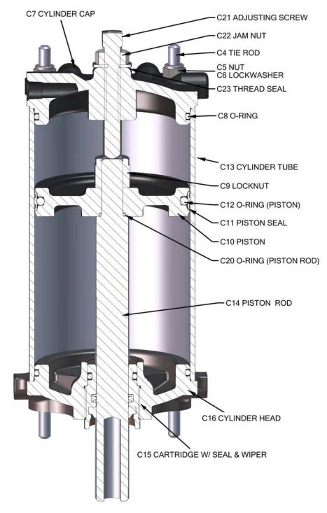
**Figure 2: Component Identification**
