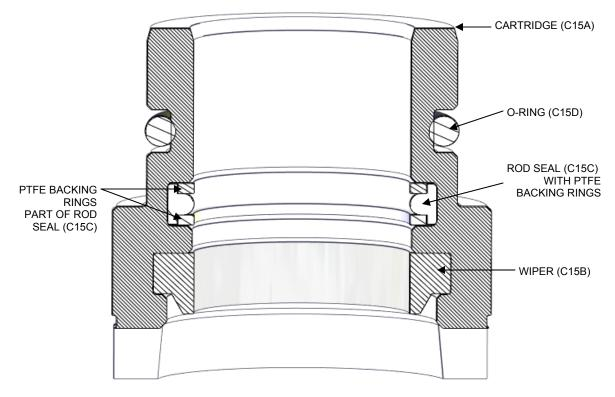
Figure 3: Cartridge Assembly (C15)
