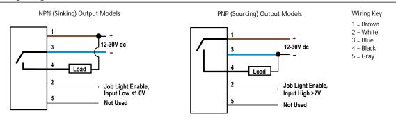
Note: Cabled wiring diagrams are shown. Quick disconnect (QD) wiring diagrams are functionally identical.
