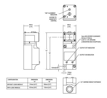
Figure 3. Dimensions for the FF models
