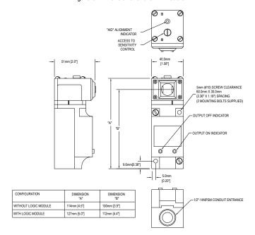
Figure 4. Dimensions for the fiber models
