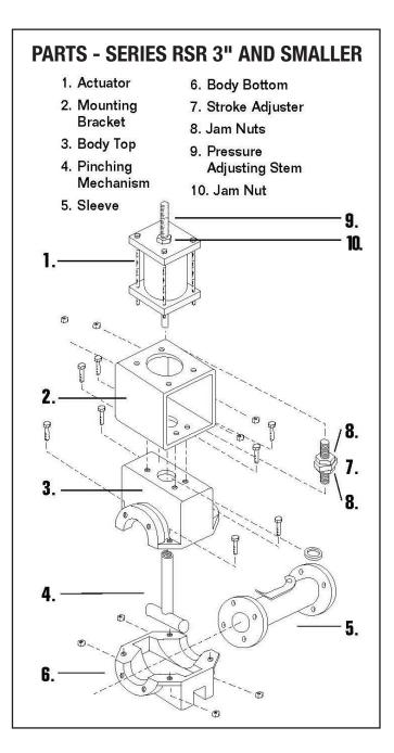
3. Tighten all flange bolts to values listed in the table on the back page. You will not overtorque the flange rubber.
