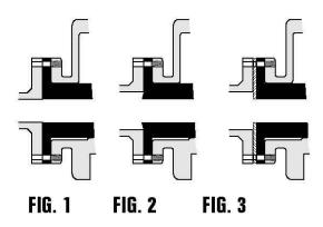
If it is not possible to match the pipe and sleeve I.D. as described above, the flanges will mate and the sleeve I.D. will protrude into the pipeline (Fig. 2). To prevent bulging and premature breaking of the Double Wall Sleeve, a steel washer must be installed as shown (Fig. 3). The steel washer should be 1/8" thick and be serrated. The washer 0.D. can be just short of the bolt holes, or it can equal the flange 0.D.
