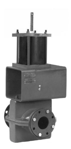
The Red Valve Series RSR Pressure Relief Valve is a bi-directional valve designed for tough slurry applications. The elastomer sleeve closes on entrapped solids in the line. The flexing action of the sleeve breaks up any sediment or build-up in the valve, which makes the Series RSR a reliable, low-maintenance pressure relief valve. A variety of elastomers are available to suit yourspecific needs.
