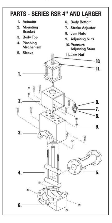
2. Be certain the valve is closed completely and not cracked open in the closed position. Operating the valve in a cracked open position can shorten sleeve life, since flow velocities are very high under these conditions.
