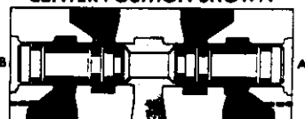
3-POSITION DUAL PRESS. PRESSURE CENTER (SPOOL ASSY. #S-08002) CENTER POSITION SHOWN
