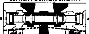
3-POSITION DUAL PRESS. PRESSURE CENTER (SPOOL ASSY. #S-08002) CENTER POSITION SHOWN
