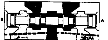
3-POSITION SGL. PRESS. CLOSED CENTER (SPOOL ASSY. #S-00004) CENTER POSITION SHOWN
