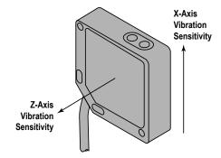
After determining the sensor direction and location, mount the sensor for the best possible vibration sensing accuracy. Mounting options in order from least effective to most effective are as follows:
