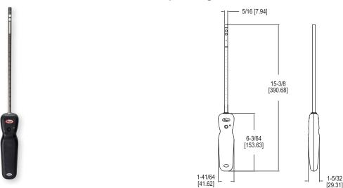
The Series AP2 Wireless Thermo-Anemometer Probe measures air velocity, air flow, and temperature when combined with Models UHH and UHH2 or the Dwyer Mobile Meter® app. In order to prevent damage to the sensing element, the probe has a protective sleeve that slides over the sensor when it is not in use. Markings on the probe allow users to know the insertion depth to obtain better accuracy when traversing the duct.
