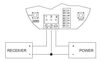
Figure 3: Voltage Output Wiring
