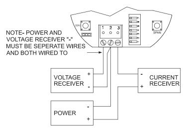
Figure 4: Simultaneous Current and Voltage Output Wiring
