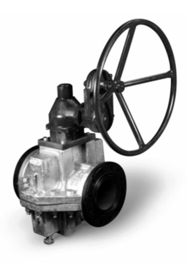
The Red Valve Series 9000 manually actuated Pinch Valve is a bi-directional valve designed for tough slurry applications. The elastomer sleeve closes on entrapped solids in the line. The flexing action of the sleeve breaks up any sediment or build-up in the valve, which makes the Series 9000 a reliable, low maintenance valve.
