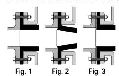
sleeve. The washer O.D. can be just short of the bolt holes, or it can equal the flange O.D. and bolt holes can be drilled through the washer.
