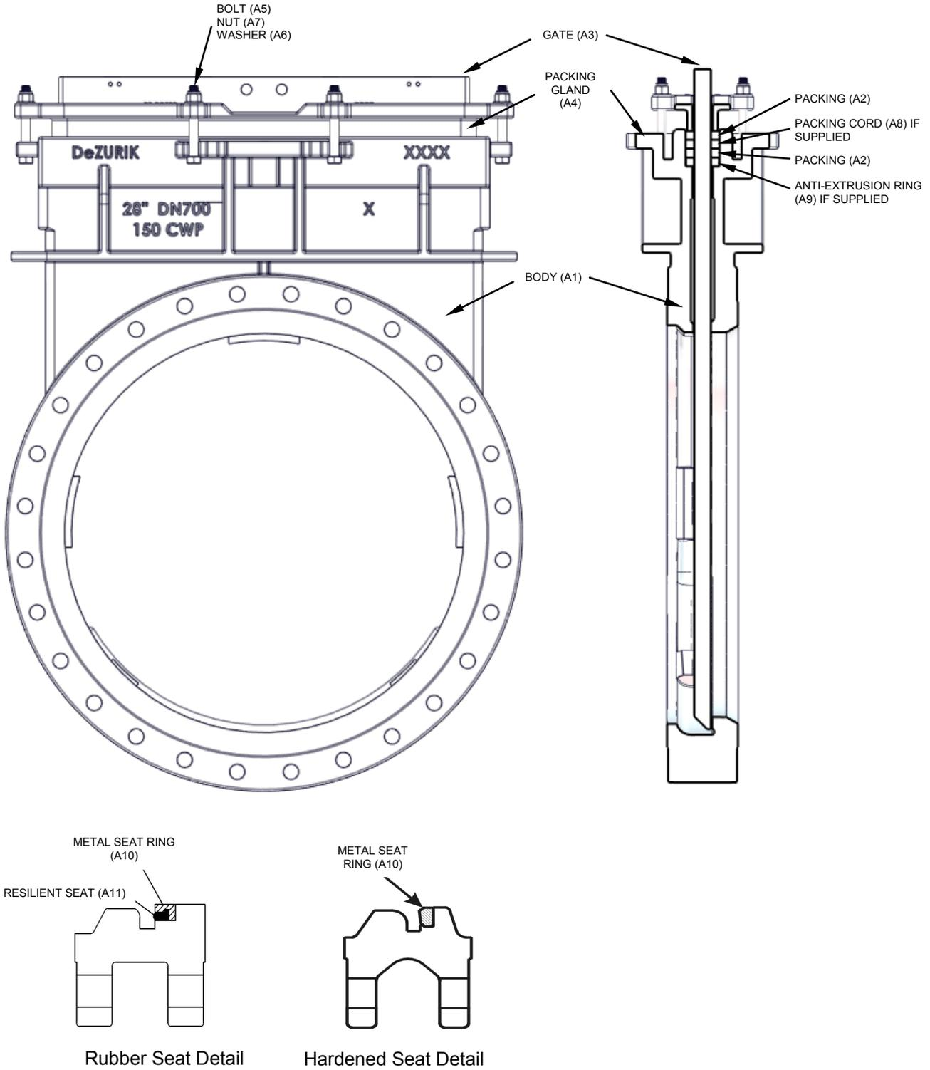
Figure 2—Component Identification
