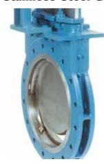
All valves are provided with 304 stainless steel guides for corrosion resistance. Gates are finish ground on both sides and edges to increase packing life. Gate guide provides rigid support for the moving gate. Gate jams at the bottom of the body hold the gate securely against the seat.
