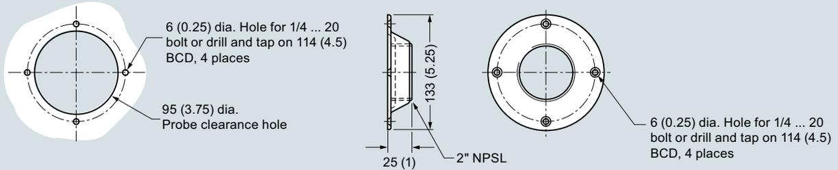
**Note:** Mounting flange supplied with probe.
