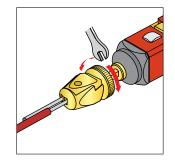
Figure 10. Applying tension to the rope (models RP-LS42F-..LE)
