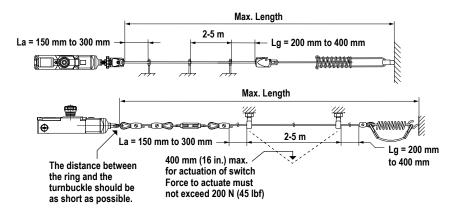
Figure 6. Assembly of Rope and Hardware
