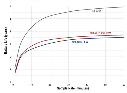
Figure 3. Battery life for the Q45VA, VT, and U Nodes
