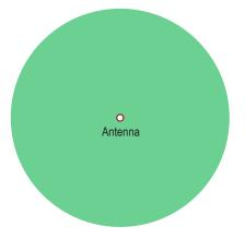
From the top view, the signal radiates equally in all directions from the antenna. For this reason, omni-directional antennas are best used for the device in the center of a star topology network.
