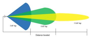
Because Yagi antennas yield narrower radiation patterns, accurately aiming a high-gain Yagi is important when setting up a radio network. The higher the gain of the antenna, the more the signal is focused along a specific plane. High-gain antennas should only be used for line-of-sight applications.
