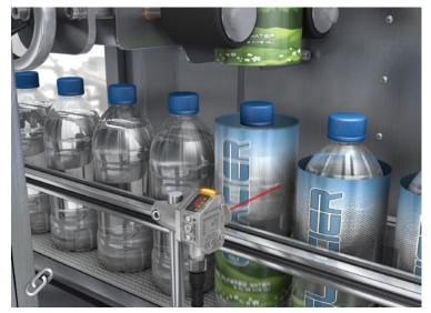
The Q4XCOD laser sensor provides greater precision and more reliable bottle detection than LED-based sensor solutions. When triggering shrink sleeve labels, increased line speeds and greater throughput are possible.
