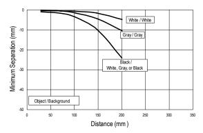
Figure 5. Minimum Separation Distance Between Object and Background
