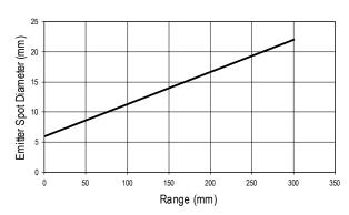
Figure 4. Typical Emitter Spot Diameter vs. Distance
