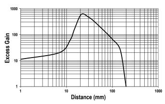
Figure 7. Excess Gain Curve with 200 mm Cutoff (based on 90% White Card)
