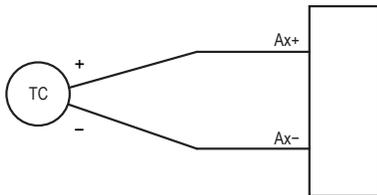
Thermocouple: When wiring the thermocouple, x is the same number. For example, a thermocouple is wired to A1+ and A1-.
