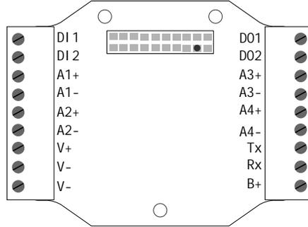
B+. 3.6 to 5.5 V dc (use for battery powered models only)
