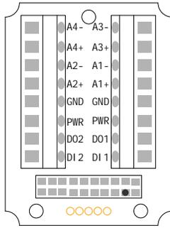
Ax+ and Ax-. Analog IN x. Analog inputs for devices requiring more than one connection, such as thermocouples or RTDs. When there is no Ax-, use Ax+ as an analog input.
