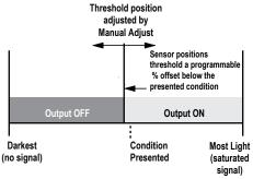
Figure 9. Light SET (Light Operate shown)
