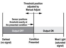
Figure 11. Calibration SET (Light Operate shown)
