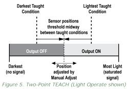
The Output ON and OFF conditions can be reversed by using the LO/DO (Light Operate/ Dark Operate) switch.
