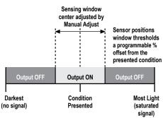
Figure 7. Window SET (Light Operate shown)
