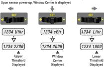
Figure 8. Upper and Lower Thresholds
