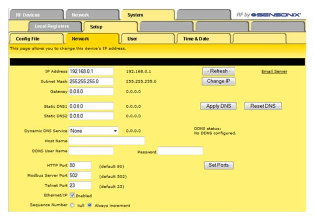
To use EtherNet/IP, the GatewayPro or DX83 Ethernet Bridge interface requires the user to enable the EtherNet/IP interface, define the EtherNet/IP registers, and save the system configuration using the *System > Setup > Config* File page.
