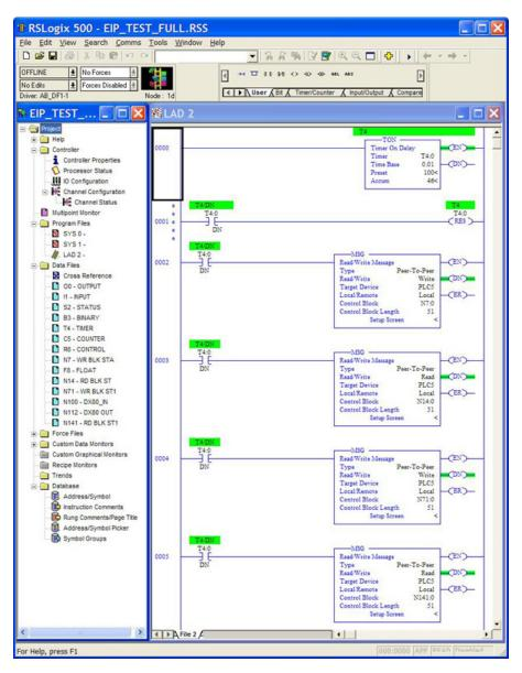
Figure 1. SLC 5 Set-up MSG. In the example screen shown, a counter is set up to activate the MSG Read or MSG Write blocks every one second. Also two write and two read MSG blocks are shown. Each MSG block can only handle up to 103 words.
