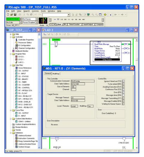
Figure 3. SLC 5 – MSG Write Setup. The SLC 5 MSG write setup instruction with multi-hop enabled is shown. Click on the 'MultiHop' tab and enter in the IP address of the DX80 Device (factory default 192.168.0.1)
