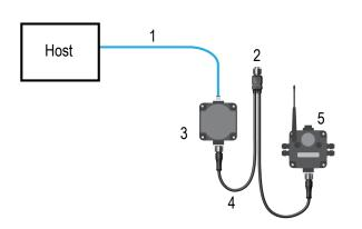
1. Ethernet crossover cable using the Modbus/TCP or EtherNet/IP communication protocol
