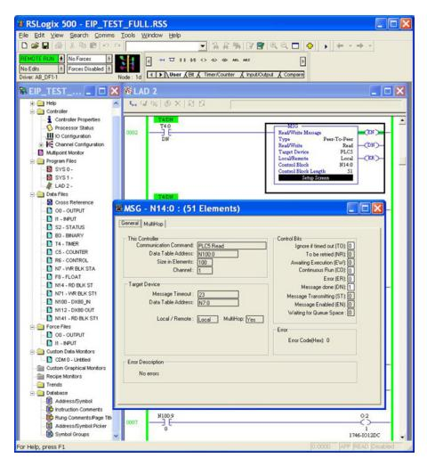
Figure 2. SLC 5 – MSG Read Instruction. The SLC 5 MSG read instruction with multi-hop enabled is shown. Click on the MultiHop tab and enter in the IP address of the DX80 Device (factory default 192.168.0.1)
